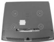
Align the four matching pegs on the back of the main unit as circled in the left picture with the four matching holes in the wall mount brackets as also marked in circles in the top pictures and allow the main unit to slide down the winding grooves in the wall mount backpack. Connect all cables coming out of the
