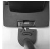
washers to hold the joint tight. For low profile customer display PD-305, the installation procedure is same. Remember to enable the +5 V DC supply in the COM port of the main unit for PD-2501, PD-2602 or PD-305 or the +12 V DC in VGA port for LM-6201.
